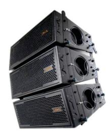
The M26LA passive modular line array source features 2-way passive (biamp) design equipped with 2×6.5 inch LF speaker with 2.5 inch voice coil mounted in a port assisted configuration allowing for increased sensitivity at the low end.
